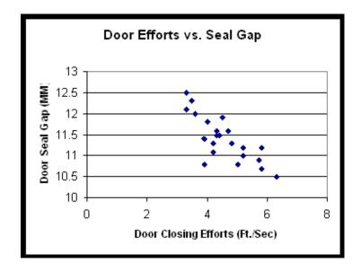
In this case, the process improvement team is analyzing door closing efforts to understand what the causes could be. The Y-axis represents the width of the gap between the sealing flange of a car door and the sealing flange on the body - a measure of how tight the door is set to the body. The fishbone diagram indicated that variability in the seal gap could be a cause of variability in door closing efforts.
